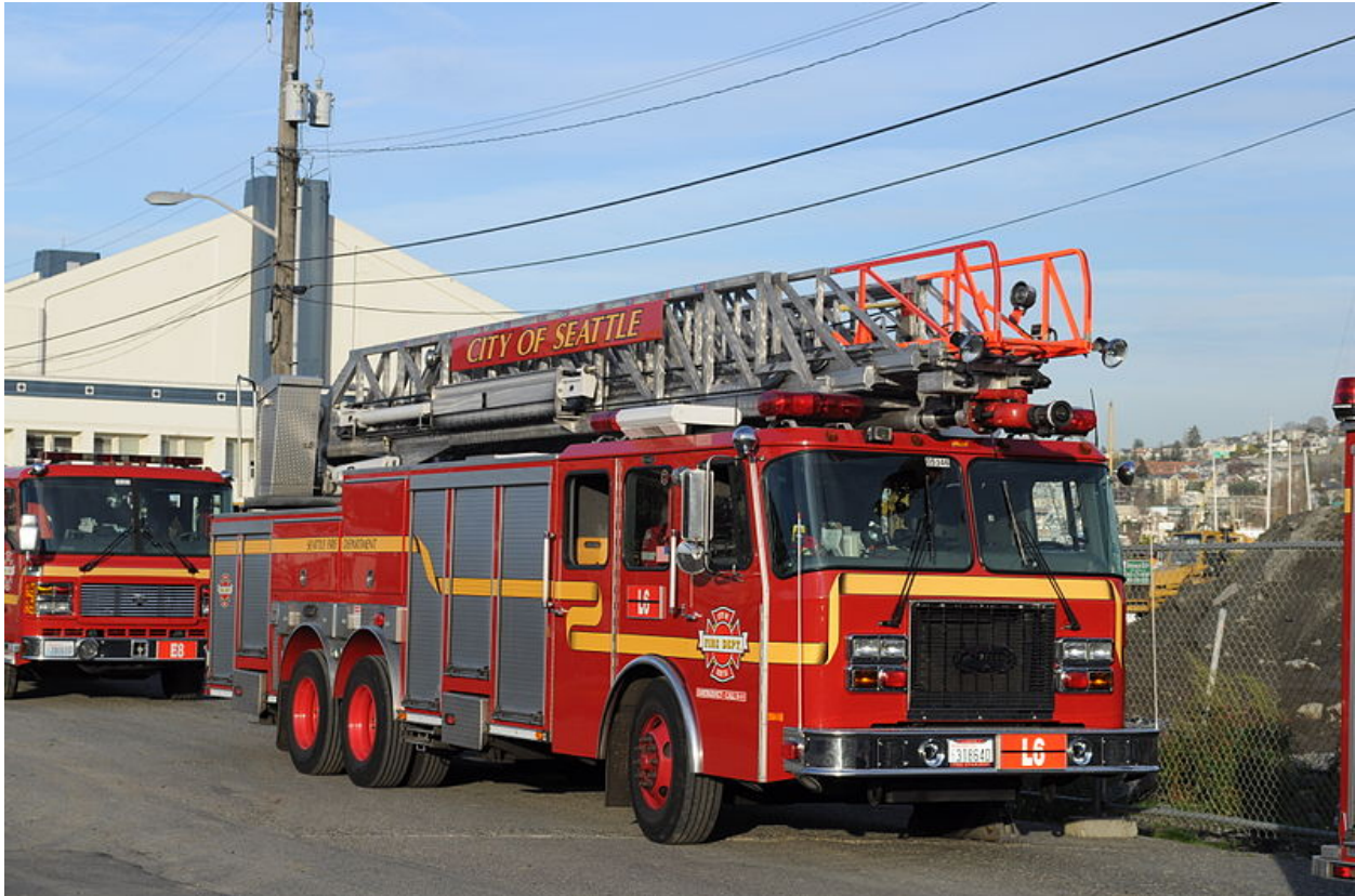
Figure 1.1 – Aerial Ladder Truck (Photo Credit: Joe Mabel)
